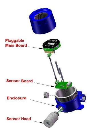
Important: Calibrate the transmitter whenever a component is replaced. But if you replace a smart sensor assembly with a sensor onboard from QEL, you don't need to recalibrate the transmitter, as all the calibration information has been stored in the smart sensor board in factory process.
