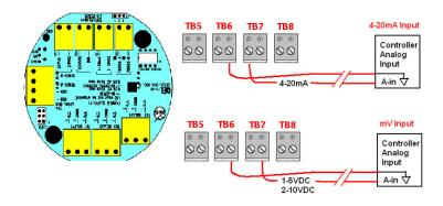
Test point mA+ and mA- on top plate board are used to measure the 4-20mA output current inline when the Q8 is working in the field.
