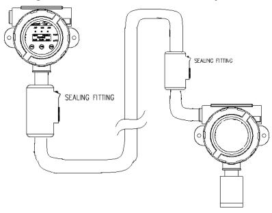
The Smart Sensor Head can be equipped with Q8 locally or remotely. For installations where the smart sensor head assembly will be mounted remotely from Q8, the max distance between Q8 and Remote Smart Sensor Head is 100 meters. The Remote Smart Sensor Head Assembly is not included in the Q8 standard package, it must be ordered separately.
