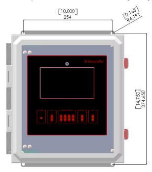
The enclosure is a NEMA 4X rated enclosure and can be wall mounted with 4 screws. To maintain the NEMA rating, it is important that the conduit opening is sealed upon installation.
