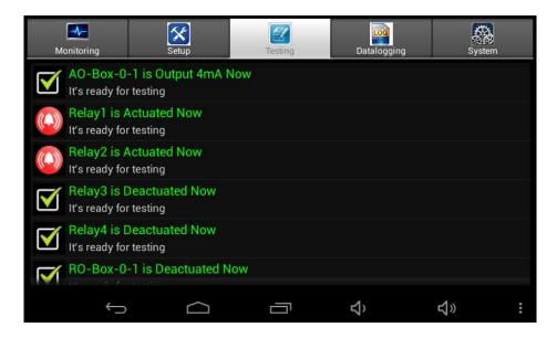
For system installation testing, it is necessary to force relay, buzzer and strobe actions.
