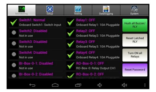
On-board switch input, on-board relay/buzzer/strobe/horn output and all remote modules are real time monitored in the screen.
